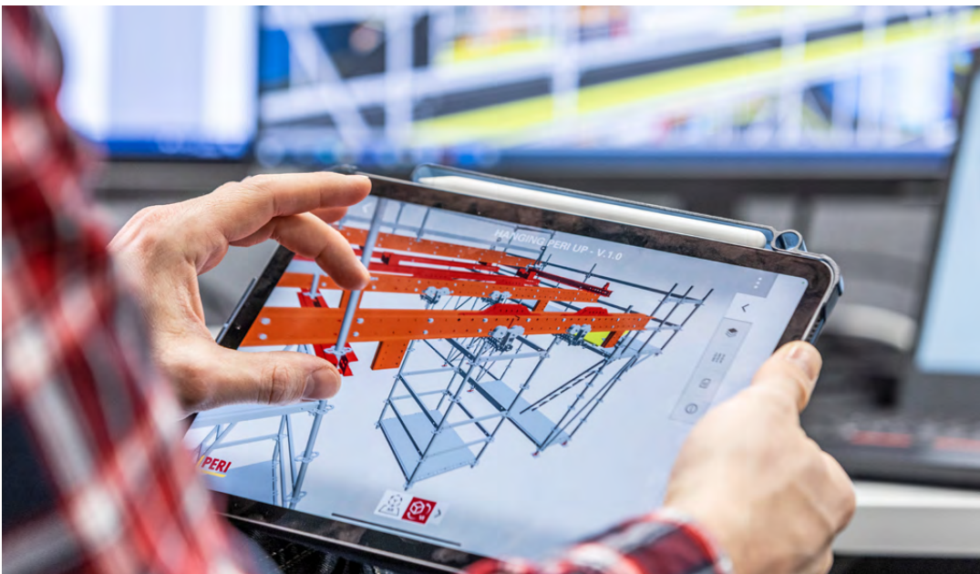
3D visualization of formwork and scaffolding projects with the PERI Extended Experience app.
